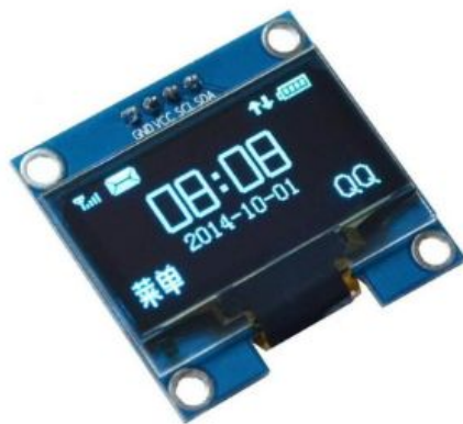
Figura 7. Display Oled 128x64
